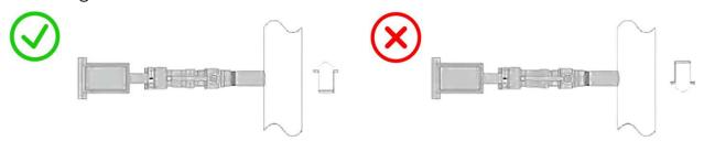
Avoid a partially empty pipe, during operation the pipe must be either completely full of liquid or completely empty
