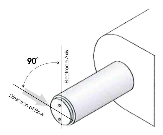
• The electrodes must be in 90° with the flow. See figure below.
